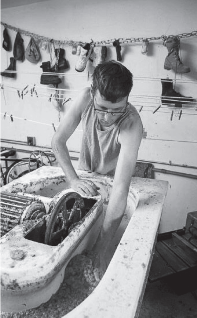
Figure 1 Nathan Lewis pictured in his Trumansburg, NY studio. Here he uses a Hollander beater to turn shredded military uniforms into paper pulp. Photograph courtesy of David Burbank.
